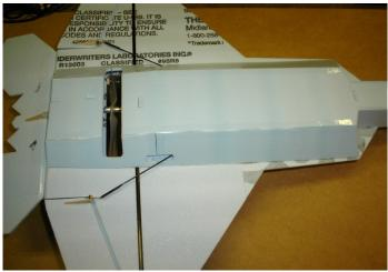
Sand a bevel on the inside of the top plate so it sits right up against the fuselage and round over the outside edges.
