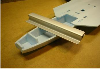
Sand the top half of the fuselage sides where it meets the bottom fuselage assembly. You don't have to worry about sanding the part where it sits over the wing.
