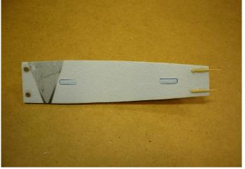
Make sure the push rod cutouts are extended to the fold line on the bottom fuselage part.
