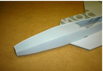
Glue motor mount, control horns and elevator servo mount in place. Flip over and sand the middle of the fuselage assembly flat.
