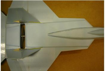
Attach a piece of velcro to the inside of the hatch area for your battery to sit. A 3s 1300 mah lipo should set at the back of the hatch area to give you the right C.G. The C.G. is where the leading edge starts to angle forward.
