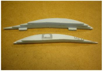
Glue the nose pieces together. Sand and shape the canopy and attach it to the top fuselage part. The nose will get shaped later.
